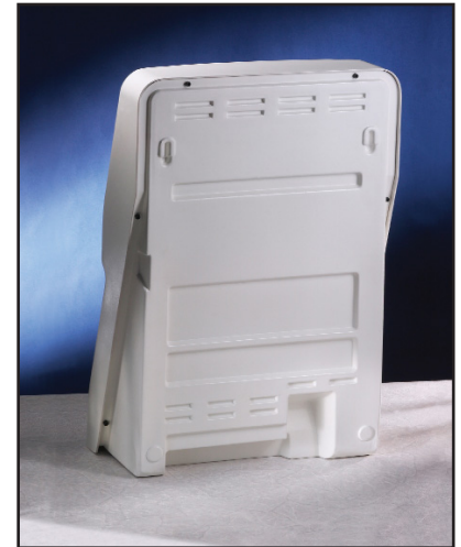
Net wall thickness of SyncStationXM rear-panel, deep-drawn corners exceeds 0.71mm (0.028"), meeting UL Std. 94 V-0 requirements. Offset touch points assure breathing room when the unit is wall mounted.
