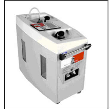
High Fluid Cart uses a two-piece lid fabricated of KYDEX® T thermoplastic alloy sheet to guard against spillage during operating-room use. Outer portion of the lid is pressure-formed and adhesive-bonded to a vacuum-formed inner lid, then sealed with a gasket.
