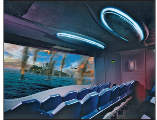
Using electric actuators to pitch, sway, and heave simulators containing from 6 to 40 seats, SimEx is able to immerse audiences into underwater adventures and faraway space flights. Yet, the simulator motion also causes excessive wear and stress to seats and side panels, and requires a high-impact, high-strength material like KYDEX® 100 sheet, a proprietary thermoplastic alloy typically enlisted by the aerospace and transportation industries.
