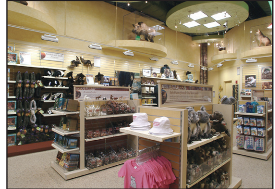
The museum store at the Smithsonian Institution's Kenneth E. Behring Hall of Mammals complements the exhibition theme using a landscape of slat wall in graduated earth tones, and three-dimensional shelving that is membrane pressed and miter folded with KYDEX® sheet in ivory colour.
