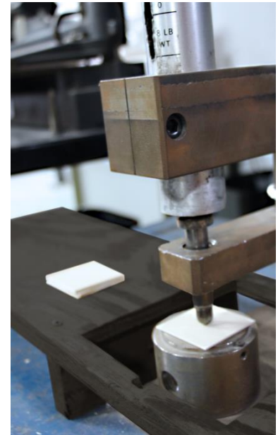
At top: Falling weight drop dart test with GE geometry: the smallest outer diameter and largest rounded metal head. At bottom: Geometries for HIC zones are stronger than ever. KYDEX ® 6523HI compared to non-HIC sheet results from Gardner Drop Dart Impact Testing.
