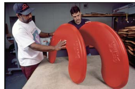
KYDEX sheet conforms to all top and side surfaces of three-dimensional substrates which, in this case, consist of doubled MDF board with injection molded Coca-Cola® logos affixed prior to membrane pressing, allowing seamless reproduction of corporate identity that resists damage.
