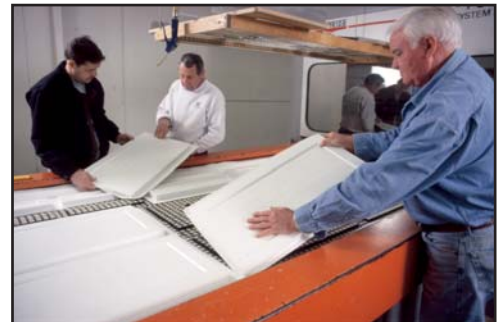
White door panels clad in Renolit film are removed from the membrane press prior to trimming. Owner John Colby on right.
